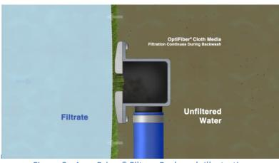
Figure 2: AquaPrime® Filter - Backwash Illustration
