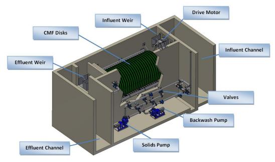
Figure 3: AquaPrime® Filter Arrangement
